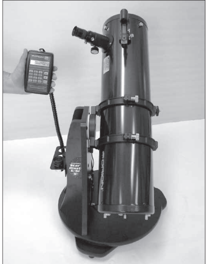
Figure 25. If you're positioned to the left of the telescope and face the direction the optical tube is pointed, the guide arrows on the Computerized Object Locator will correspond exactly with the direction you should move the telescope to pinpoint the selected object.
