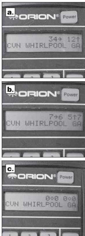
Figure 26. This sequence of pictures illustrate how the Computerized Object Locator's guide arrows look as you are finding a celestial object. (a) When the optical tube is aimed far away from the object's location, there will be a number (from 10 to 179) to the left of the guide arrows. (b) When the scope is aimed close to the object, each guide arrow will display a number on its immediate left (from 0 to 9) and immediate right (from 0 to 9); the number on the left is whole number increments, while the number on the right is in increments of tenths. This helps in making small movements to the telescope to pinpoint the object's location. (c) When the guide arrows display "0.0 0.0", the object will be within the field of view of the telescope (with a 25mm or longer focal length eyepiece).
