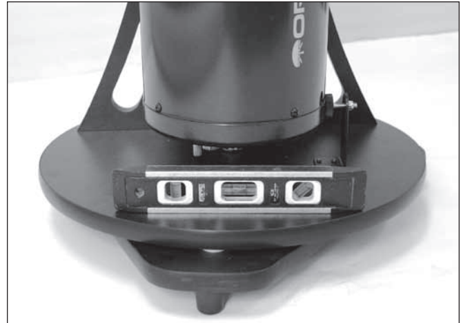
Figure 23. Place a carpenter's level on the altazimuth base as shown. Add shims under the three feet as needed so that the base stays level through a 180-degree rotation in azimuth. Once the vertical stop is set, the base does not need to be level to function properly.
