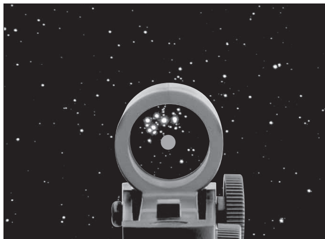
Figure 19. The EZ Finder II superimposes a tiny red dot on the sky, showing right where the telescope is aimed.
