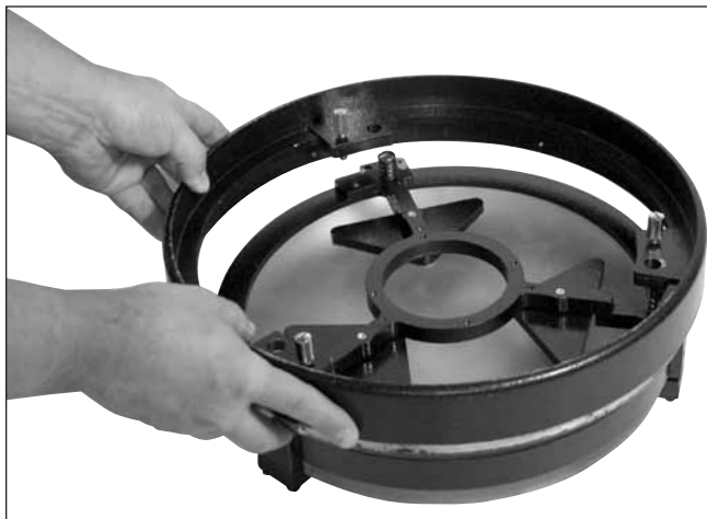
Figure 18. Lower the rear end ring onto the mirror cell so that the threaded shafts pass through the end ring, and the end ring rests on the springs.
