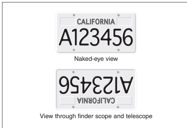
Figure 40. The view through a straight finder scope and reflector telescope is rotated 180°. This is true for the XX12 and its finder scope as well.
