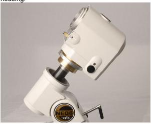
25. Replace the RA taper thrust bearing and polar scope collar on to the RA shaft. Tighten the collar just sufficiently to remove any play in the RA shaft. Lock the 4 grub screws in the collar
