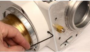
Remove 4x M6 socket cap screws from the RA worm housing.
