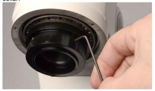
8. Using grips loosen the polar scope mounting collar. Protect the surface using thick card. An alternative to grips is to use an automotive oil filter wrench.
