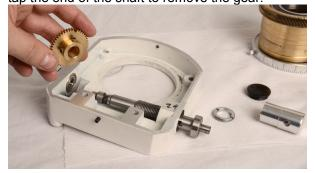
19. Temporarily place the 47 tooth pulley on the worm shaft and check the shaft shoulder is above the pulley face by 1.0mm or more. Loop a belt around a 47 tooth pulley and slide the worm back into position. Gently tighten the 2 grub screws with longer grub screw against the shaft flat.
