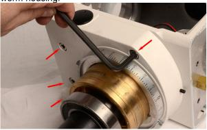
14. Remove the RA worm wheel assembly from the RA shaft. Note the position and number of any plastic shim washers.
