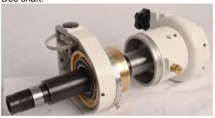
31. Carefully feed the belt through the slot in the casting while pushing the Dec shaft assembly in to position and replace 4 x M6 socket head screws and leave just finger tight. Final worm-wheel mesh adjustment can be carried out last.
