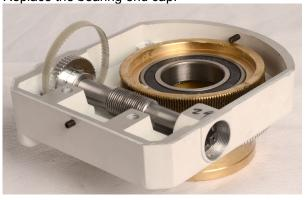
21. Replace the RA worm wheel assembly on to the RA shaft, checking that the shim washers are correct.
