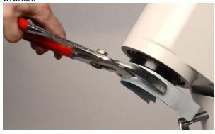
9.Remove the collar and ensure the taper thrust bearing does not fall off the end of the RA shaft on to the floor. Place it in a plastic bag to keep it clean.
