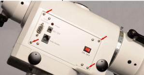
2. Remove 2 socket cap screws from each motor plate. Withdraw the motors from the housing. Make a note of which motor is RA and which is Dec.
