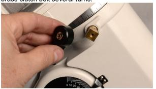
11. Withdraw the RA axis shaft assembly from the main housing. Take care to hold on to the RA taper thrust bearing. It may be necessary to use a soft faced mallet to gently tap out the shaft. Note the position and number of any plastic shim washers.
