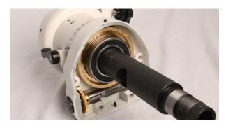
6. Unscrew the polar scope and place to one side. Remove the 3 screws from the polar scope index ring/cover.
