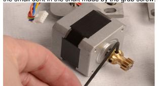
35. Fit the 12 tooth pulley on to the motor. Temporarily place the motor on the plate assembly and check the motor pulley is positioned centrally to the idler rollers. Gently tighten the 2 grub screws
