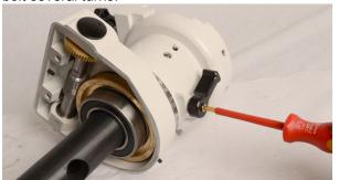
27. Remove the worm housing from the Dec shaft.
