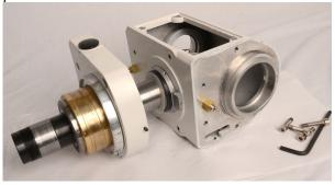
15. Loosen the RA setting circle thumb screws and lift the worm housing from the wheel. Remove the RA worm bearing end covers using
