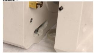
23. Replace 4 x M6 socket head screws and leave just finger tight. Final worm-wheel mesh adjustment can be carried out last.
