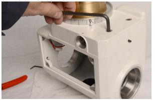
24. Replace the RA shaft assembly in to the lower housing.
