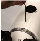
5. Withdraw the Dec axis shaft assembly from the main housing. Take care to hold on to the Dec taper thrust bearing. Place it in a plastic bag to keep it clean. It may be necessary to use a soft faced mallet to gently tap out the shaft. Note the position and number of any plastic shim washers. Place the Dec axis to one side.
