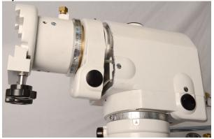
32. Replace the Dec end cap and counterweight shaft. Tighten the cap just sufficiently to remove any play from the Dec axis. Tighten the 3 x grub screws.
