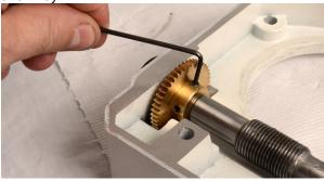
17. Using the optional bearing nut removal tool remove the slotted nut from the worm housing or alternatively use circlip pliers.
