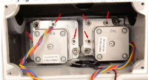
42. Connect the motors and polar illumination led to their respective sockets on the control board.
