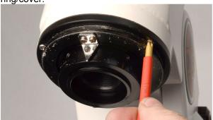
7. Slacken 4 grub screws in polar scope mounting collar.
