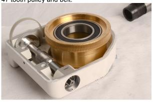
30. Fit the Dec worm housing assembly on to the Dec shaft.
