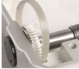
20. Replace the wheel in to the worm housing and replace the slotted nut. Lightly tighten the nut just enough to remove any axial play in the worm. Replace the bearing end cap.
