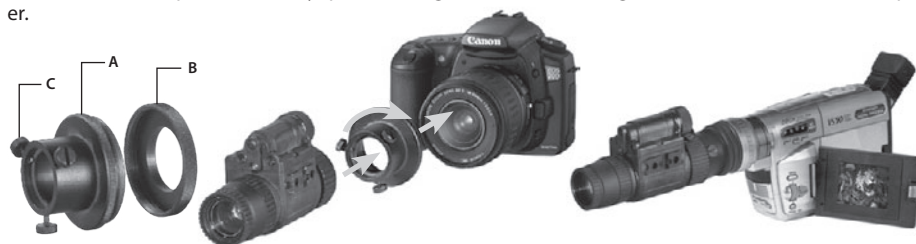
FIGURE 3-11. MOUNTING A CAMERA/ CAMCORDER TO THE N-14
