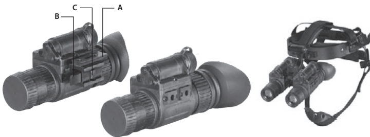
FIGURE 3-7. MOUNTING THE N-14 TO A DUAL BRIDGE
