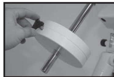
Figure 16: Install the counterweight
