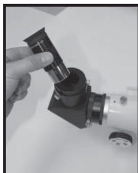
Figure 23: Insert the eyepiece
