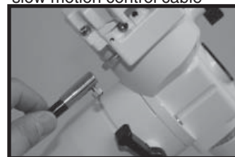
Figure 14: Attach the DEC slow motion control cable
