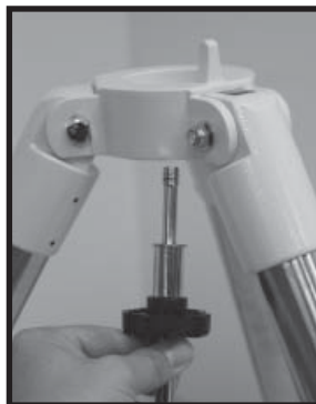
Figure 5: Installing the mount locking knob and shaft
