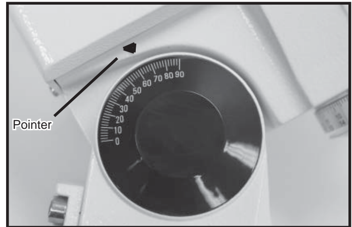
Figure 29: Latitude Scale with pointer
