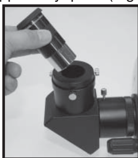
Figure 25: Insert the eyepiece
