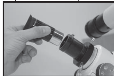
Figure 21: Insert the 26mm eyepiece
