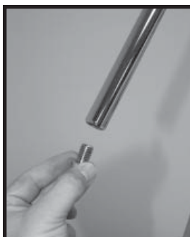
Figure 15: Remove the safety nut
