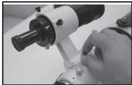
Figure 20: Attaching the viewfinder bracket
