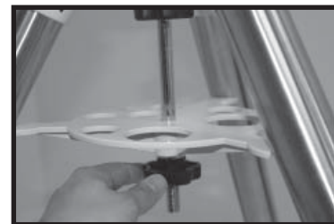
Figure 8: Tightening the spreader lock knob
