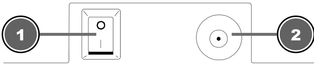
Illustration 3: DC connection socket for coaxial/barrel connector
