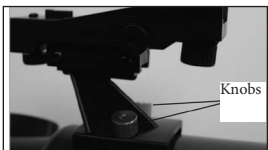
Fig. 9b: Unscrew mounting knobs and attach viewfinder. Replace knobs and tighten to a firm feel.
