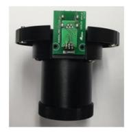
Insert two brass washers between the USB Bridge Board and the PoleMaster USB port. Insert the small locking screws. Push the USB Board down and tighten the screws.
