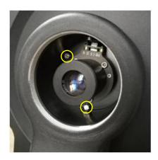
Rotate the PoleMaster to a proper position. Lock it by evenly tightening three Mounting Plate Locking Screws clockwise.
