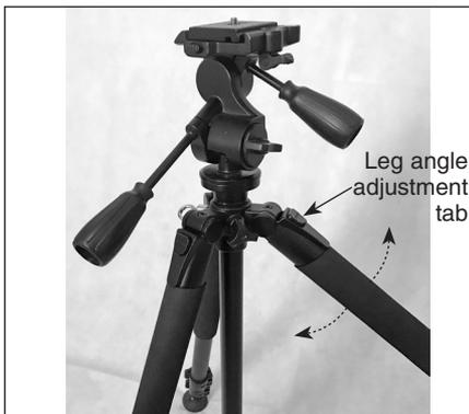
**Figure 2.** Press the leg angle adjustment tab and lever the leg up or down to one of four position angles.
