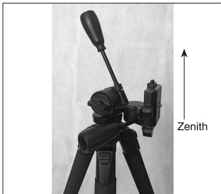
**Figure 4.** Pointing your instrument to the zenith is possible by mounting it “in reverse,” so it points up along with the long pan handle.
