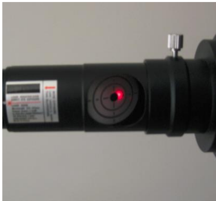
Figure 10: The primary mirror is not yet collimated.
